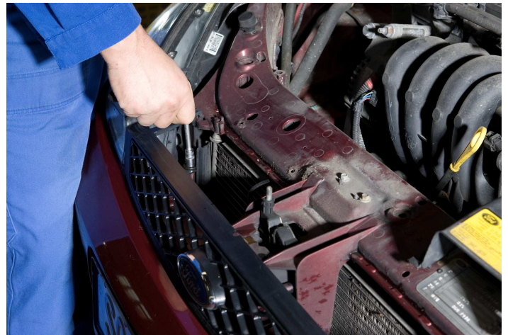
First, the grille is removed. In the case of the Ford Focus, this is in two sections!
