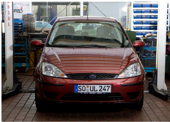
The Ford Focus 1 with series-production headlights before conversion to DynaBeam directional headlights from Hella.
